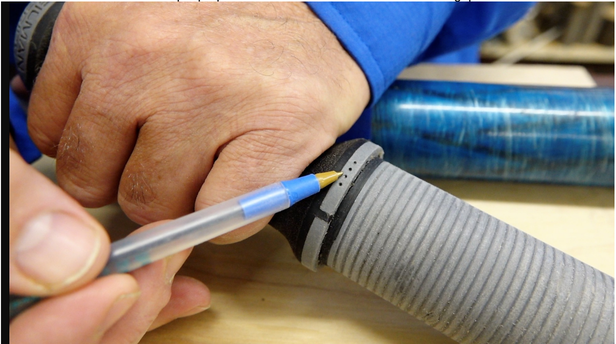
Indexing line (the top of the oar blade) inline with the 2nd indexing/clocking dot.
